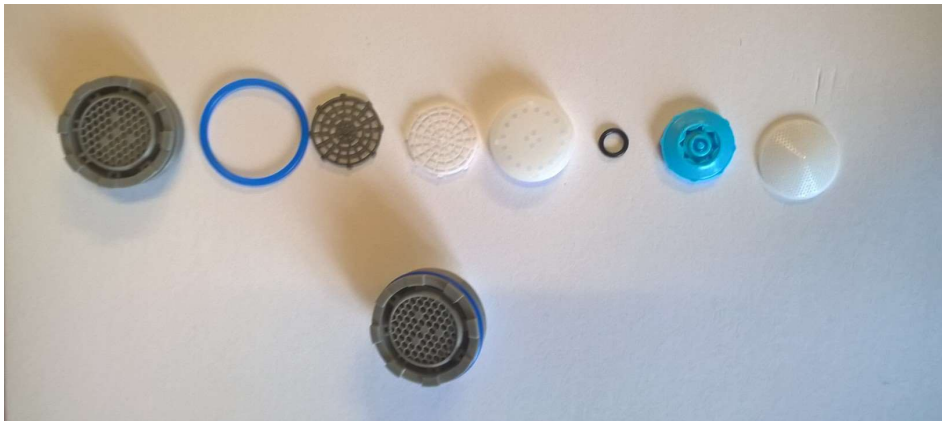
Fully dismantled flow straightener.
