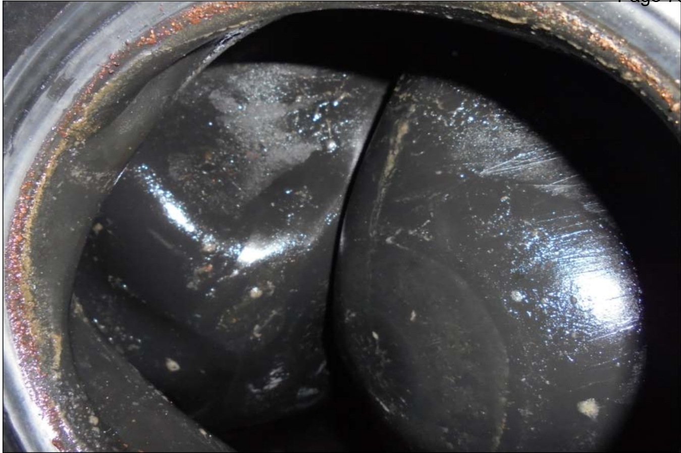
Fig 2 Trade water (expansion vessel internal bladder)
