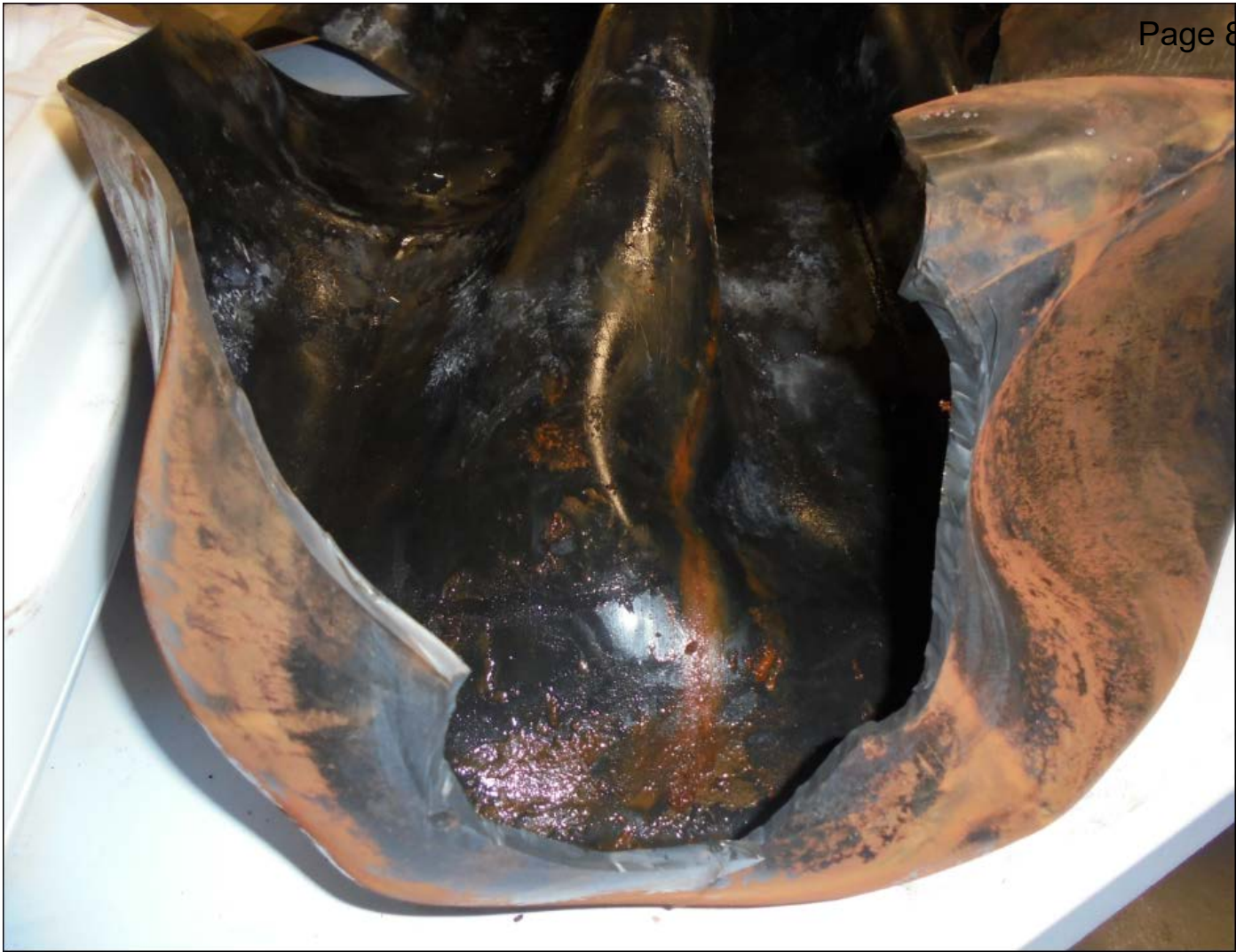
Fig 5 Trade water (expansion vessel internal bladder)
