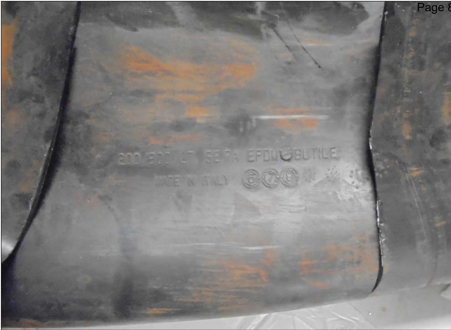
Fig 7 Trade water (expansion vessel internal bladder material)
