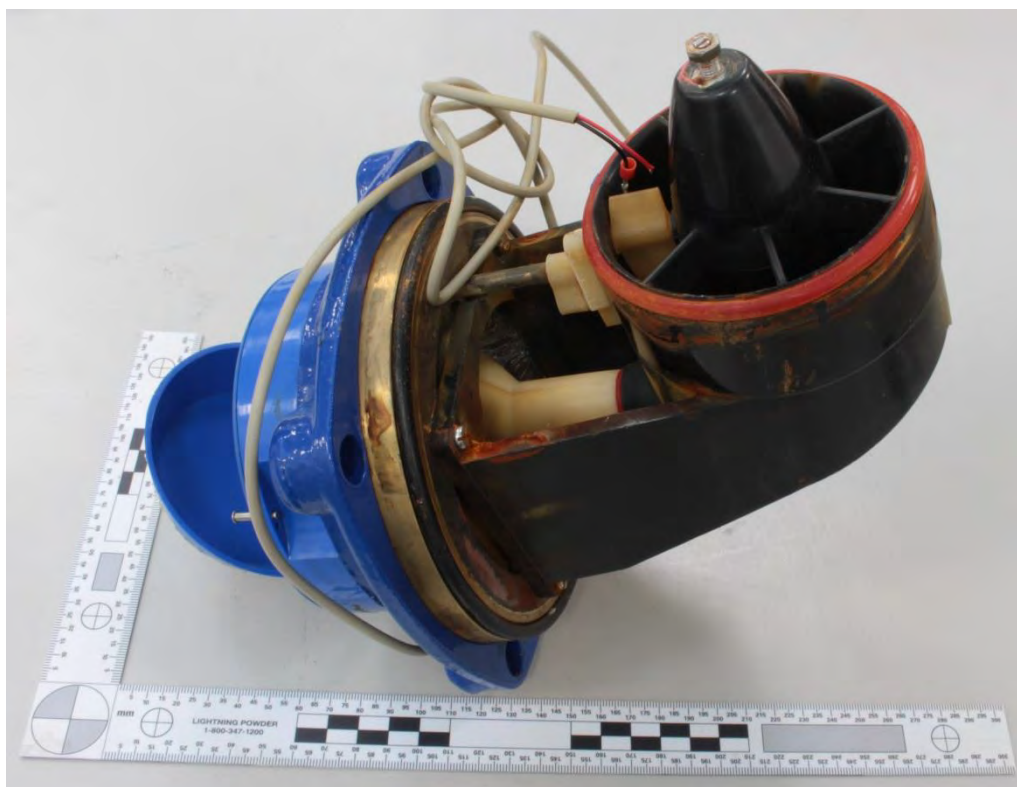
Figure 2: Water meter removed showing transferred red/brown corrosion products on the brass body.
