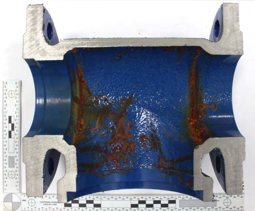
Figure 4: Overview of sectioned valve body showing corrosion products and paint blistering on internal surfaces. Note orange peel texture to paint layer.
