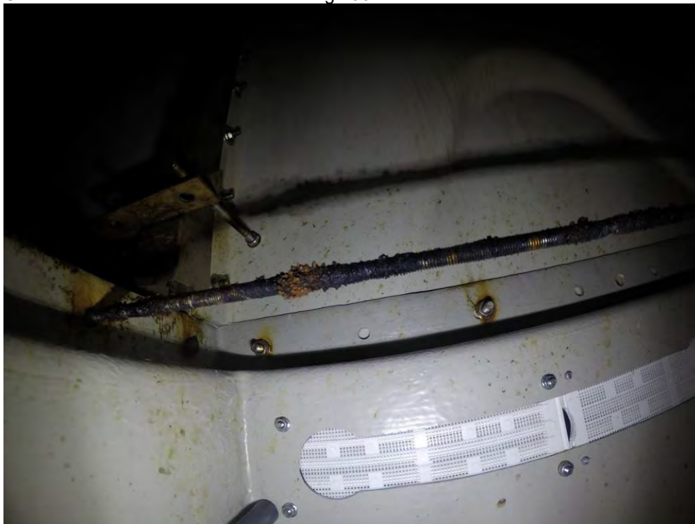
Corrosion of internal stainless steel image 002
