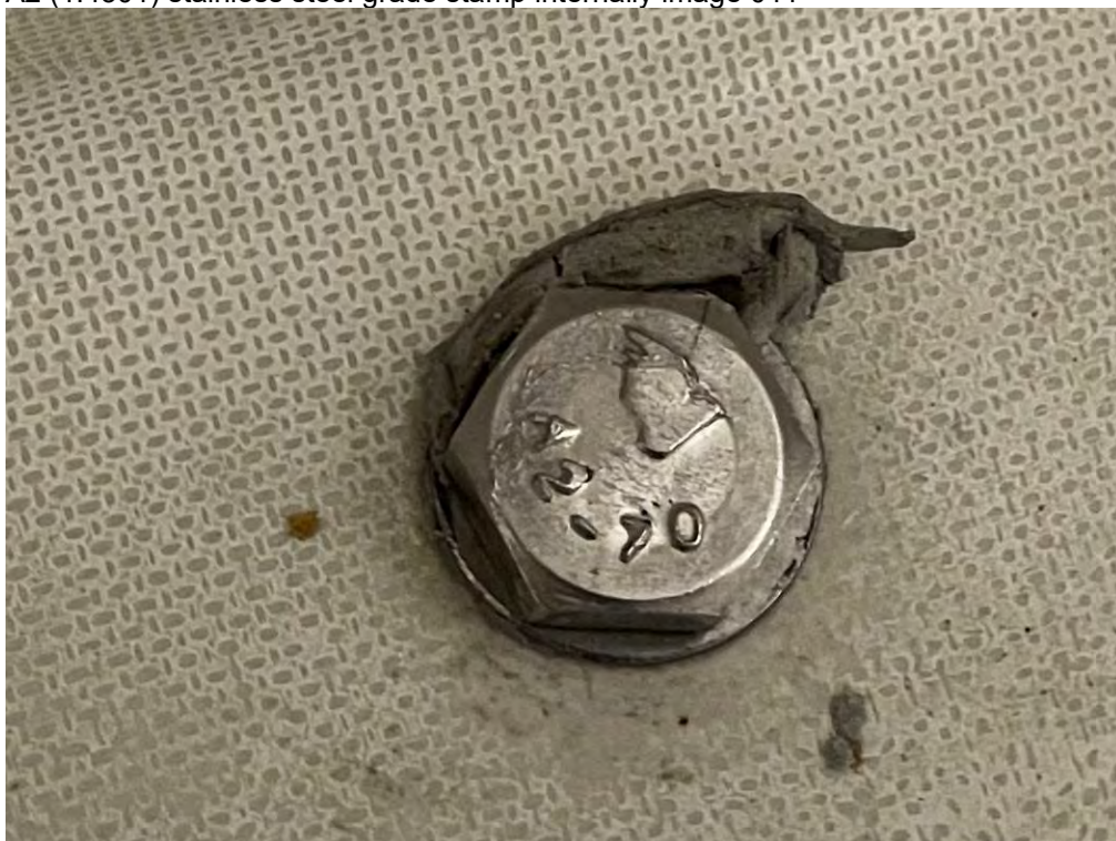
A2 (1.4301) stainless steel grade stamp internally image 011
