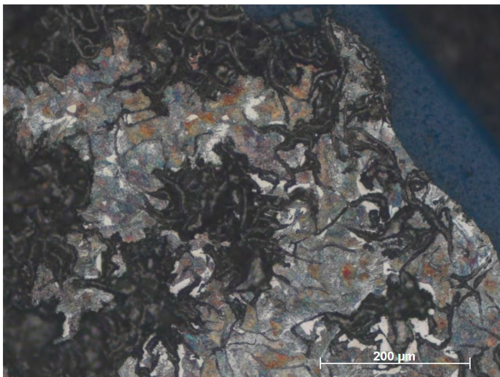
Figure 9: Corrosive attack around graphite flakes beneath paint layer. Note relatively thin paint layer.
