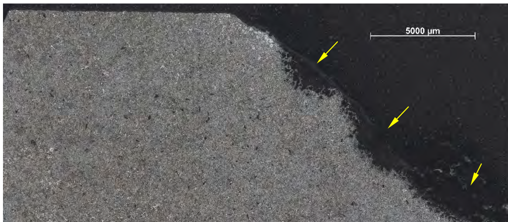
Figure 7: Optical micrograph showing section through geometry change near flange with corrosive attack typical of graphitic corrosion.
