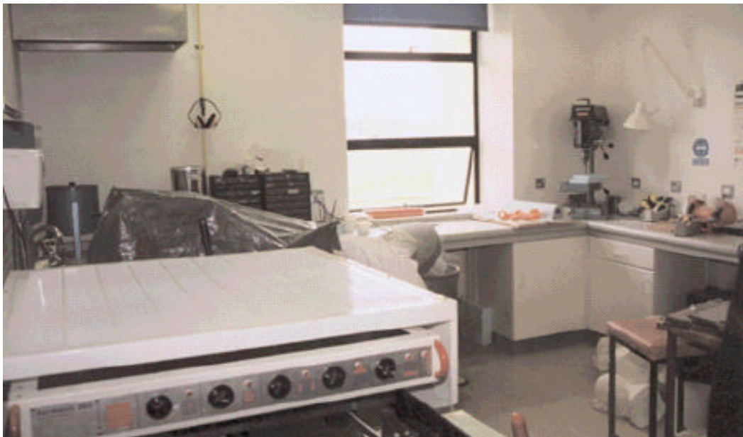
Mould room workshop showing profile machine, low temperature alloy smelting area with extract hood.
