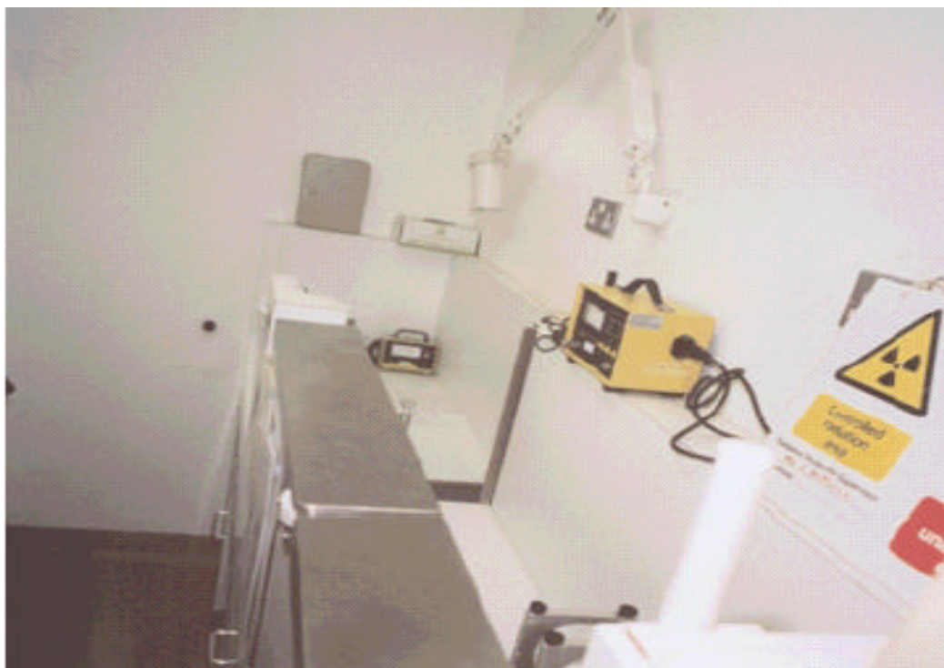
Sealed source store showing shielded workstation
