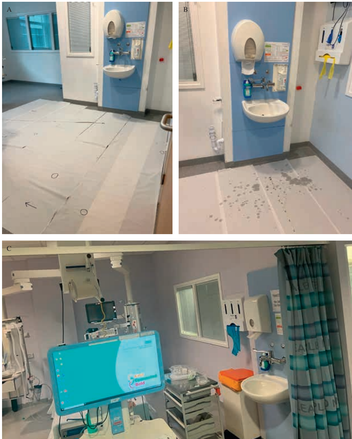
Figure 1. (A) Water from a running tap can splash some distance away from the sink, highlighted by circles on the paper towels on the floor. (B) Water can splash from undertaking hand hygiene, again highlighted by wet paper towels on the floor. (C) A typical intensive care unit patient bed space with equipment situated around a handwash basin.
