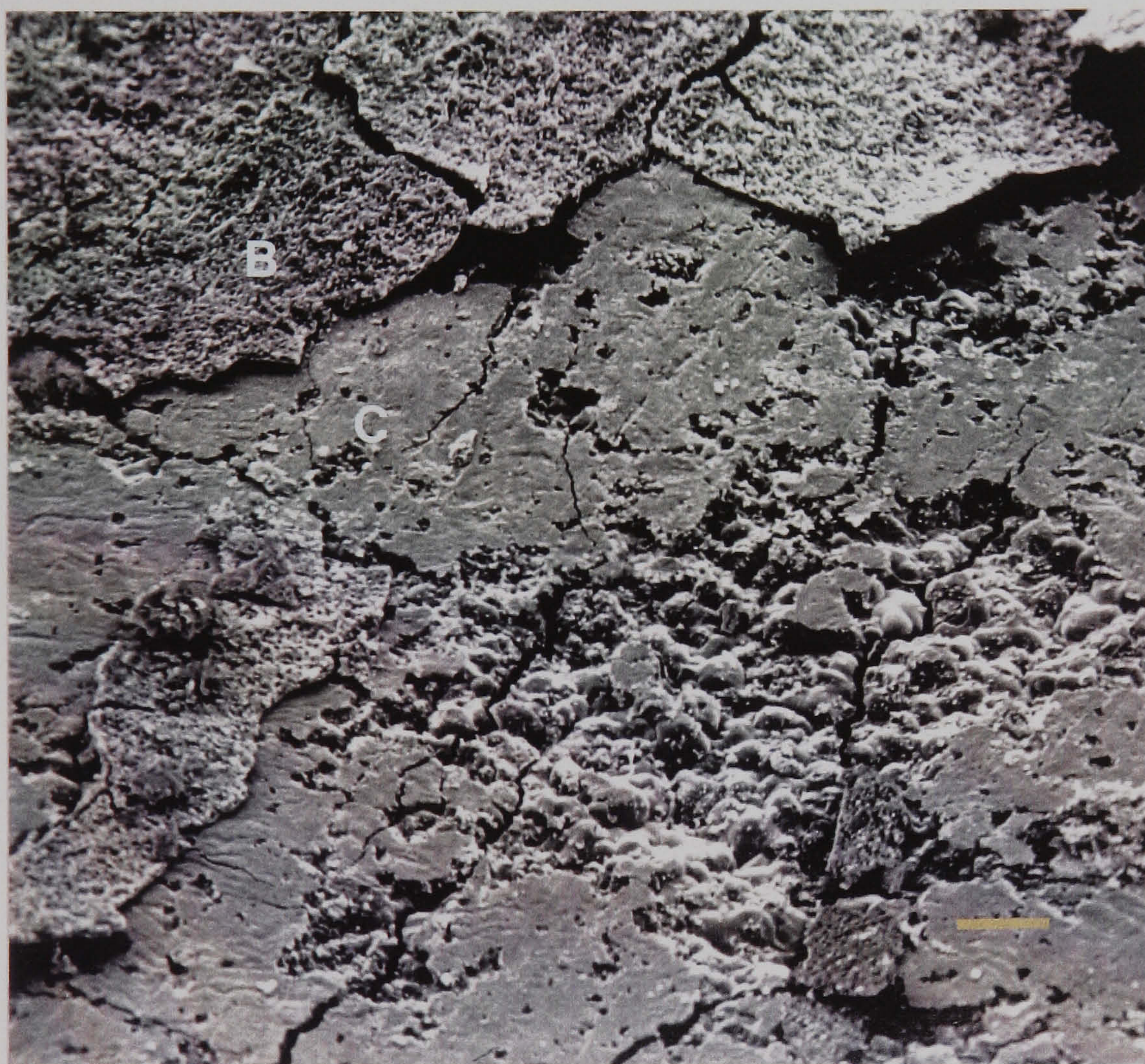
Figure. 3.4 SEM of the surface of the copper tube removed from the Glasgow Royal Maternity (Marker bar denotes 10 \mu\text{m} ; C denotes the copper surface and B denotes the biofilm layer).
