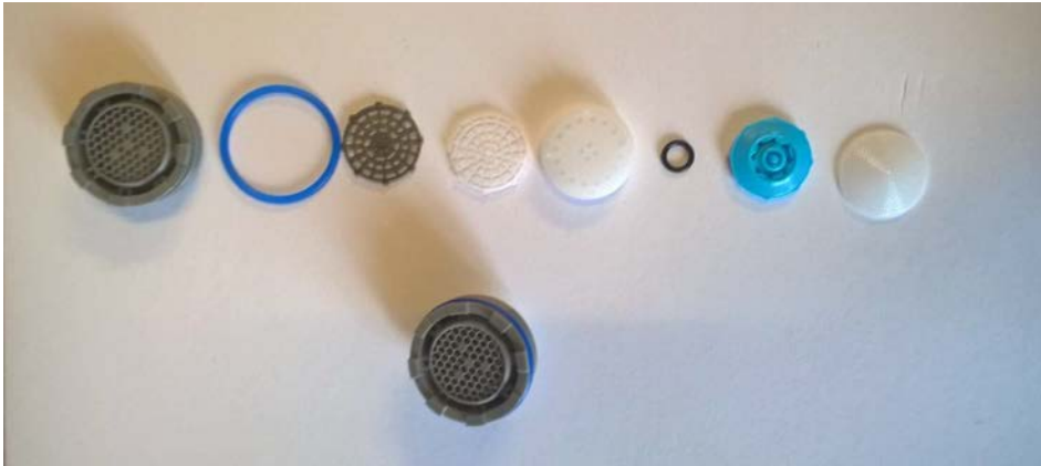
Fully dismantled flow straightener.
