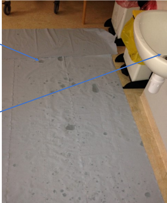
Figure 44. Splash zone as demonstrated using blue paper placed on the floor whilst someone has washed their hands in an intensive care unit (JW personal photo).
