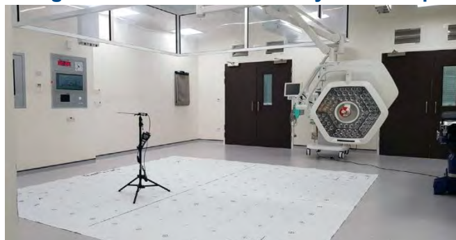
Figure 13: UCV 1m air velocity test set-up
