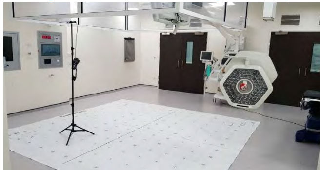
Figure 12: UCV 2m air velocity test set-up
