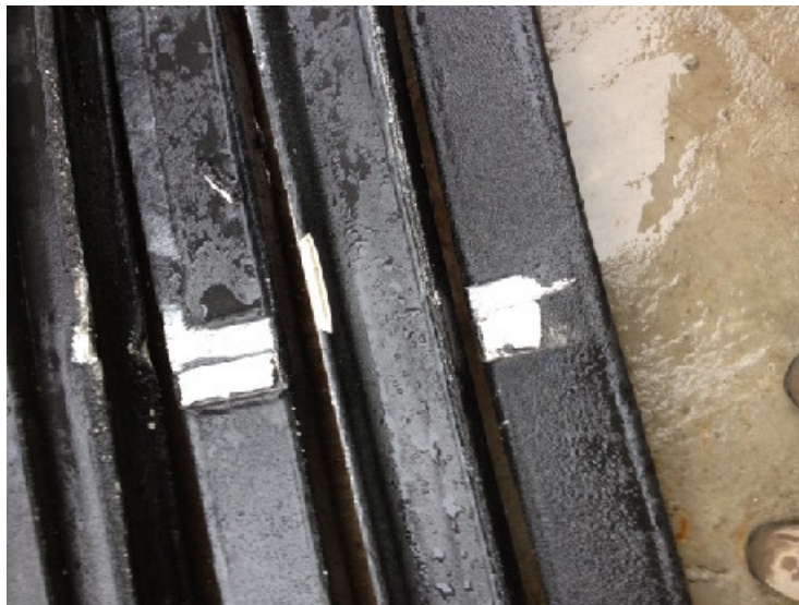
Photo 2 – Damaged intumescent cover.
